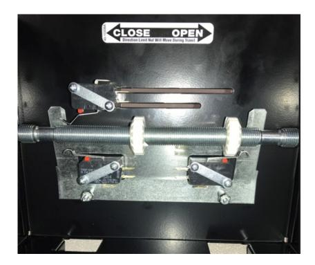
Please note, this change does require a slightly different mounting pattern; because of this, the units being produced with this temporary limit switch will have an additional set of holes drilled into the electrical box/frame. The temporary, rounded switches will utilize the pairs of upper holes closest to the limit shaft. Limit switch kits are not impacted by this change.
